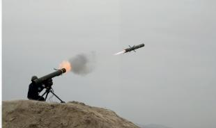
**OMTAS** is a medium-range anti-tank weapon system that is effective against armoured threats on the battlefield. Its Imaging Infrared Seeker permits day and night use, and in all adverse weather conditions.
