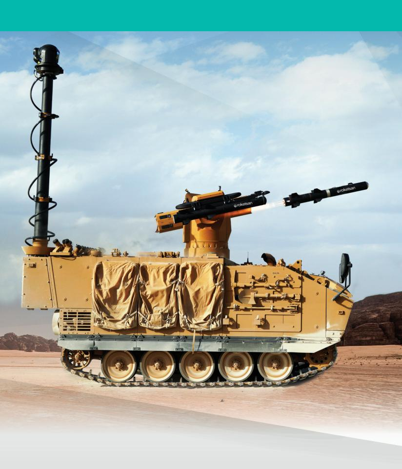
**Tactical Missile Launching System [TMLS]** is a stabilised turret system that can be used both while stationary and mobile due to its high mobility, its 360° rotation and its ability to be controlled from inside the vehicle.
